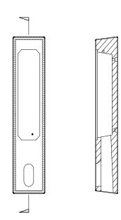
The Multi Purpose Control Pillar consists of a preformed concrete post with a large covered recess to contain a connection panel if required. Cables are brought into the recess via conduit inside the post, thus rendering the station completely weatherproof. Insulated terminal panels may be fitted and shunts or resistors are available. Identification can be supplied to customer requirements as an optional extra. The Large aluminium face plate is opened by a "drop key" device for added security.
