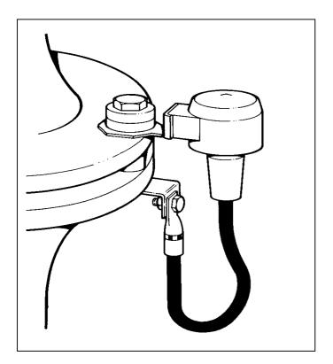
Potential hazards caused by such an incident in an area classified as "Hazardous" (Zone 2) due to the possible presence of an explosive atmosphere, can be avoided by the use of an Explosion-proof Spark Gap type SG4. The spark gap is connected in a parallel across the insulating flange and, since the connection is made using a flexible
