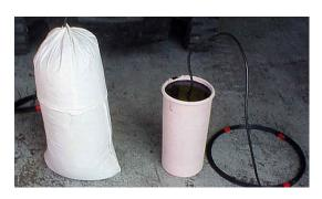
This half cell comprises a terracotta hand made container housing copper sulphate crystals and copper electrodes. Unique semi permeable design ensures excellent electrode/earth interface connection under most conditions. Under extremely high resistivity conditions the use of low resistivity back fill is recommended.
