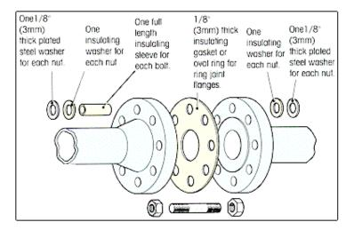
Insulating gasket manufactured from reinforced phenolic. Insulating sleeve manufactured from phenolic. Insulating washers manufactured from reinforced phenolic.
