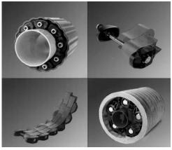
Ductile iron, concrete, metal as well as plastic pipes may be hydrostatically sealed within walls to hold up to 20 psig. Electrical or telecommunications cables may be sealed within conduit as they enter vaults or manholes. The annular space between carrier pipes passing through casings may be sealed against the entry of water, soil or backfill material.
