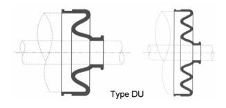
End Seals are individually designed to accommodate all types of pipe and carrier / casing differentials.
