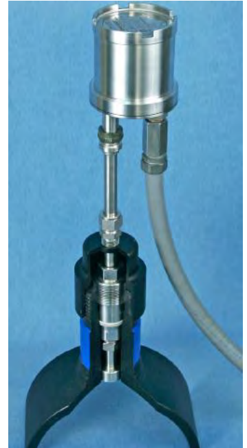
MS2600E direct mounted to a retrievable probe
